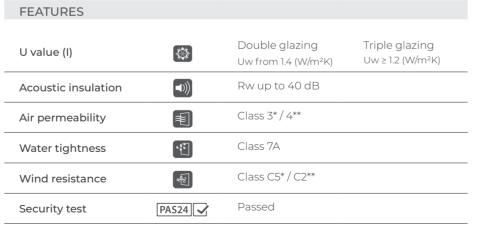
Double glazing Ug=1.0 / Triple glazing Ug=0.7 (I) Two sashes 5 m x 3 m
